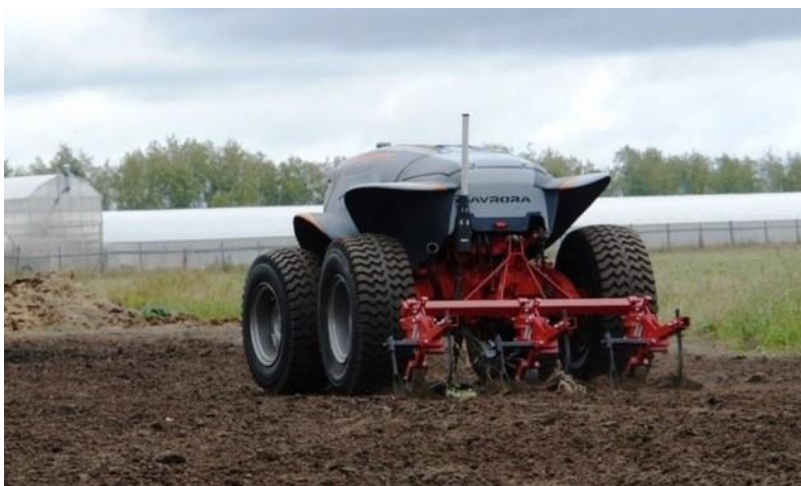
Soil tillage by the autonomous system AgroBot (Source: aurora-robotics.com)
